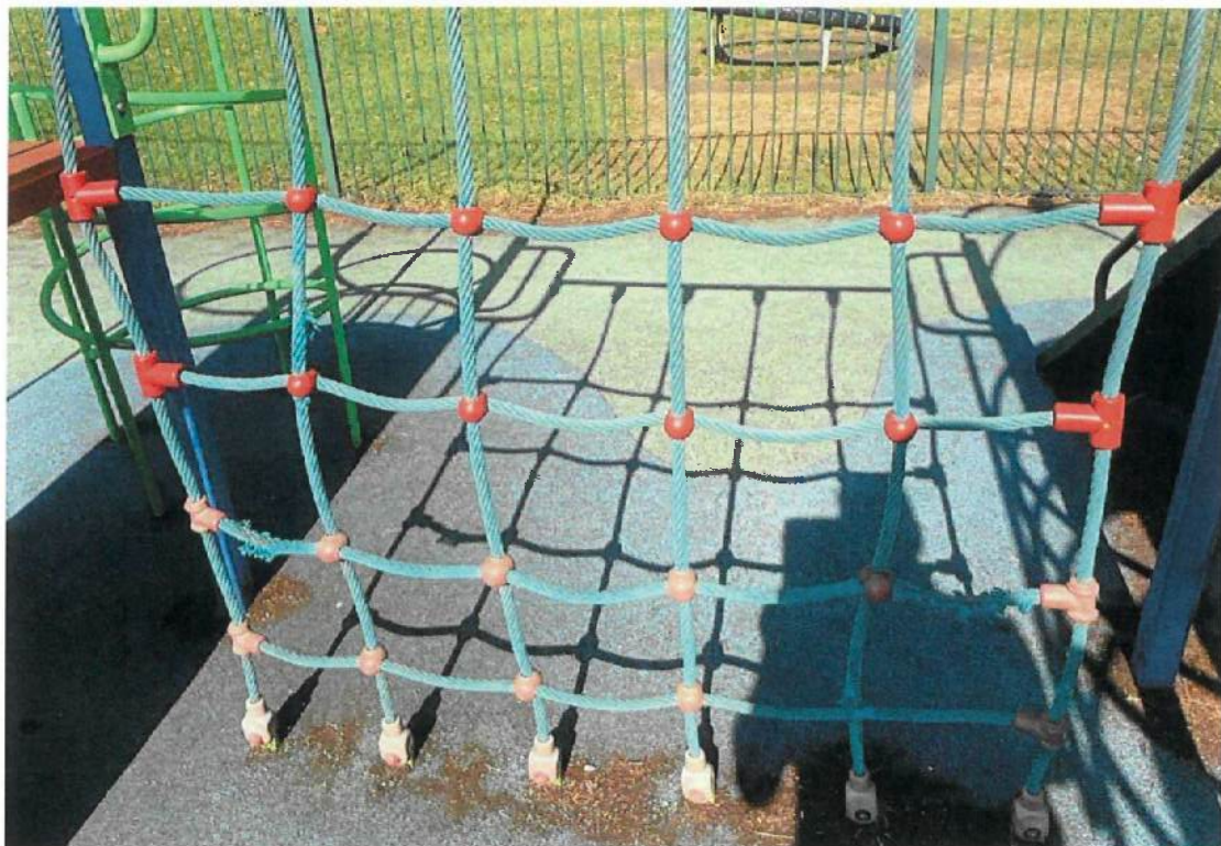
Sections of the rope cargo net showing exposed inner wires
