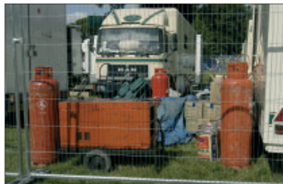
Figure 12: Example of poor storage – LPG cylinders with other combustibles
